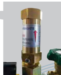
Safety Valve (Discharge Device of Abnormal Pressure)
