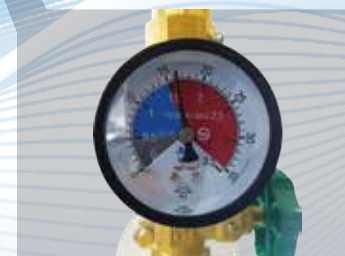
Gas Pressure Gauge
